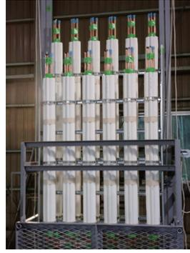
Vertical piping unit for refrigerant
